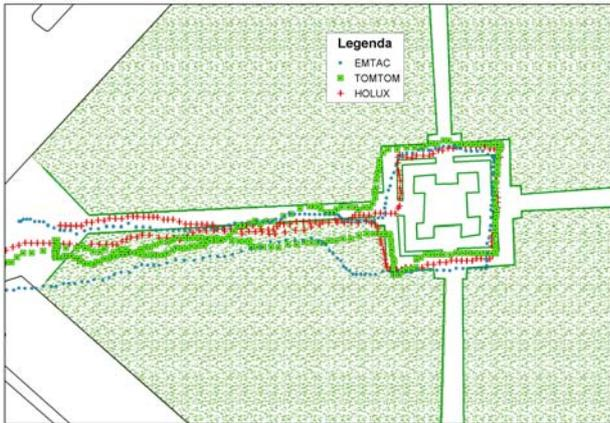
Figure 13 – Tracks using GPS receivers among trees
