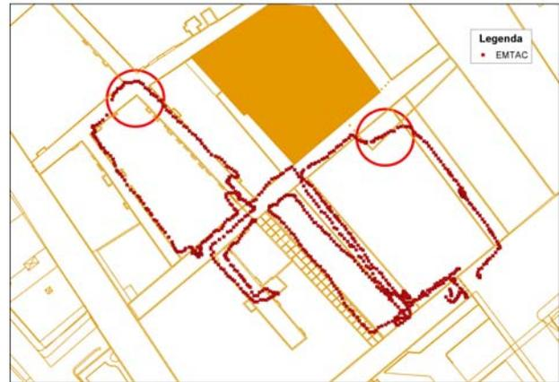
Figure 10 – A track using the EMTAC receiver
