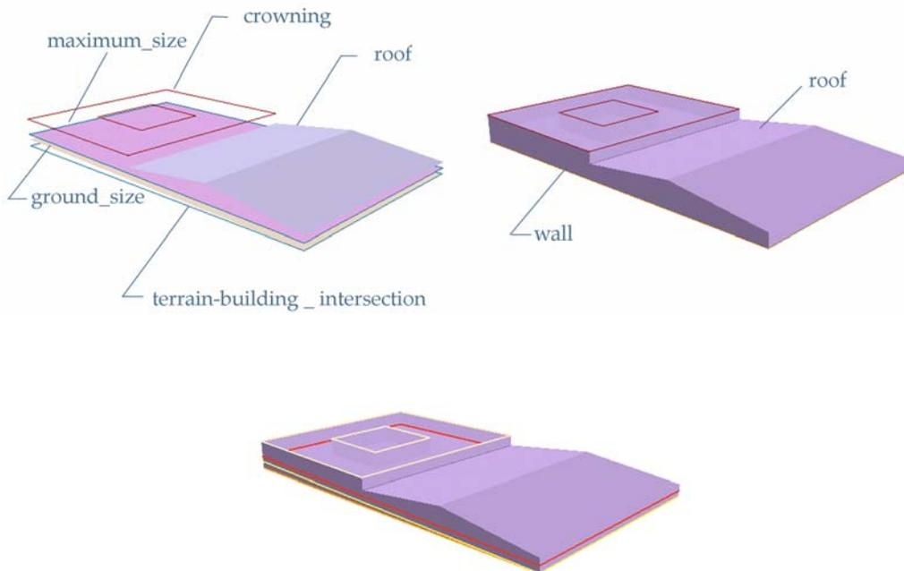
Figure 2: Components of an edifice.
